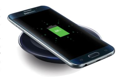
charging base, and a second induction coil in the portable device takes power from the electromagnetic field and converts it back into electric current to charge the battery. The two induction coils in proximity combine to form an electric transformer.
