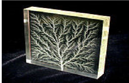
High voltage breakdown within a 4" block of acrylic creates a fractal Lichtenberg figure
